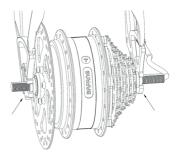
5. Mount the 2mm washer on both sides of the frame.
