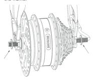
6. Tighten clockwise M12 flange nuts with open spanner at both sides of the motor. (torque requirement: 47-60N.m.)
