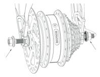
7. Mount the shaft end sheath on both sides of the shaft ends.
