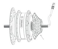
Mount first the 27.5mm washer in cable outlet side and the stop pin into on the shaft.
